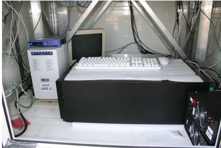
Figure 2.3: Pi2 computer controlling nightly data acquisition is located in the lower part of the ASAS dome
