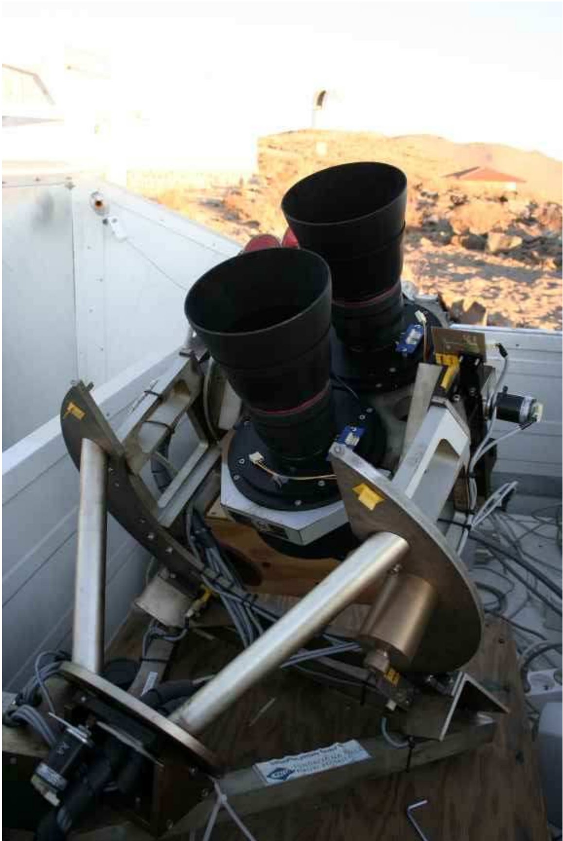
Figure 2.1: Prototype in LCO, two cameras on single mount in ASAS dome
