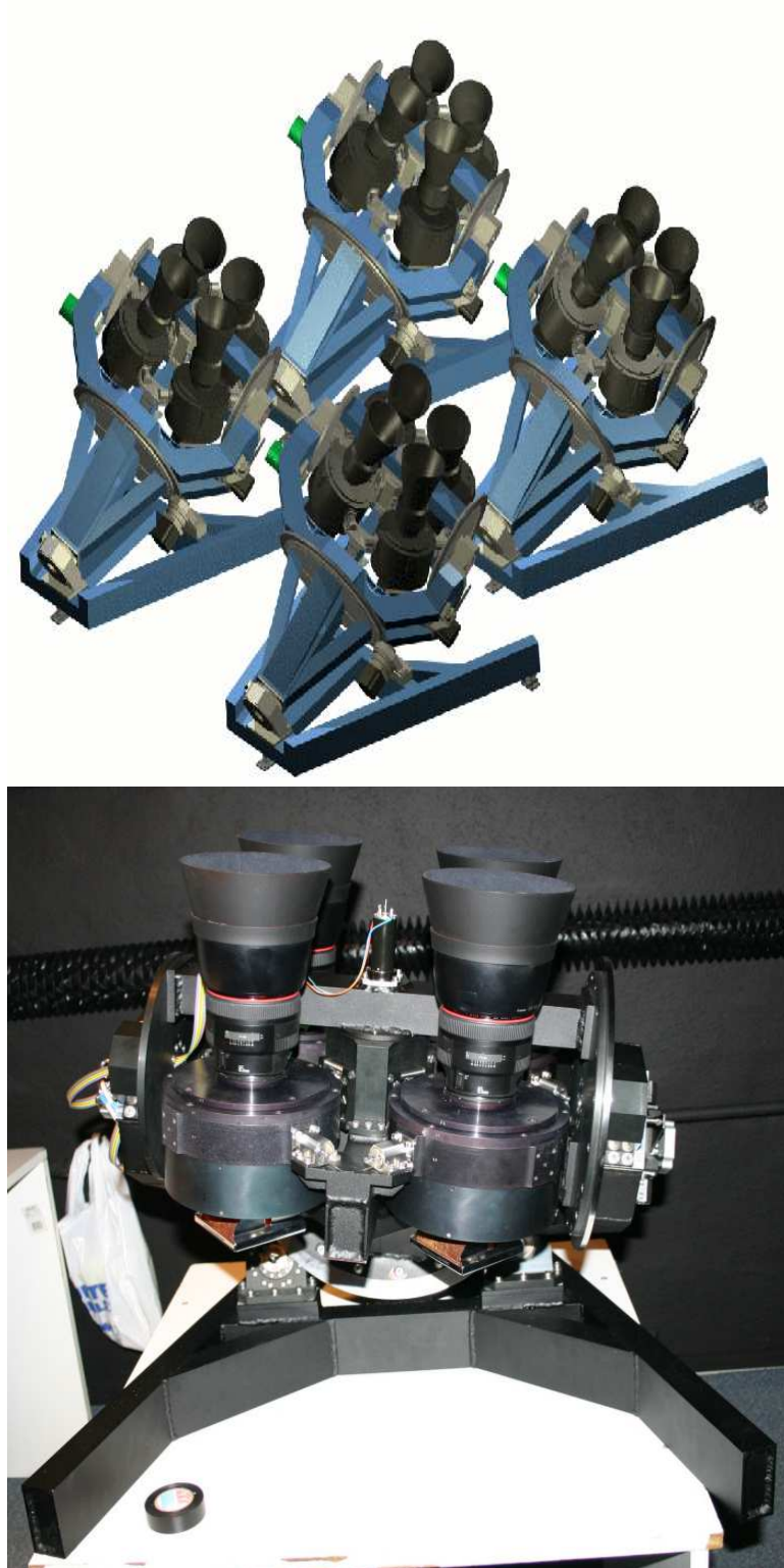
Figure 2.8: Design of new mount for full "Pi of the Sky" system (upper plot) and fully assembled mount in reality (lower plot)
